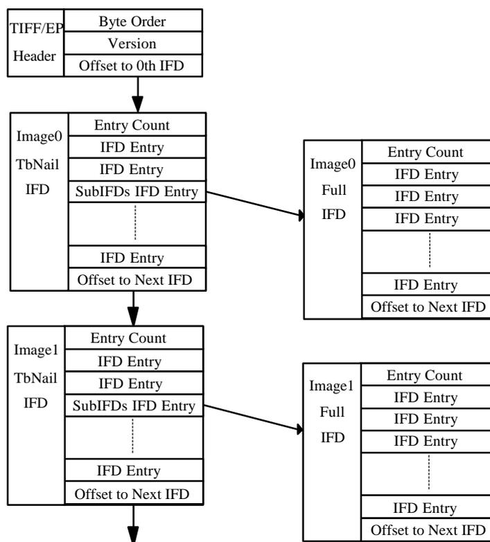
Figure 3 — TIFF/EP Encoding structure with image chaining
