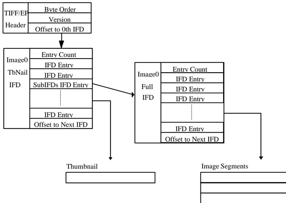
**Figure 2 — TIFF/EP Encoding structure with treeing**
